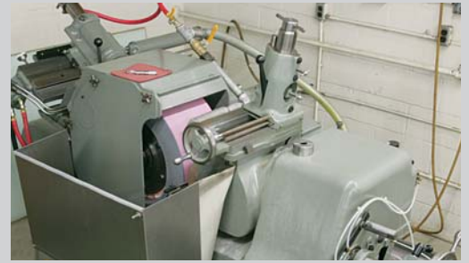
Cincinnati centerless grinder with 12" wide wheel.
