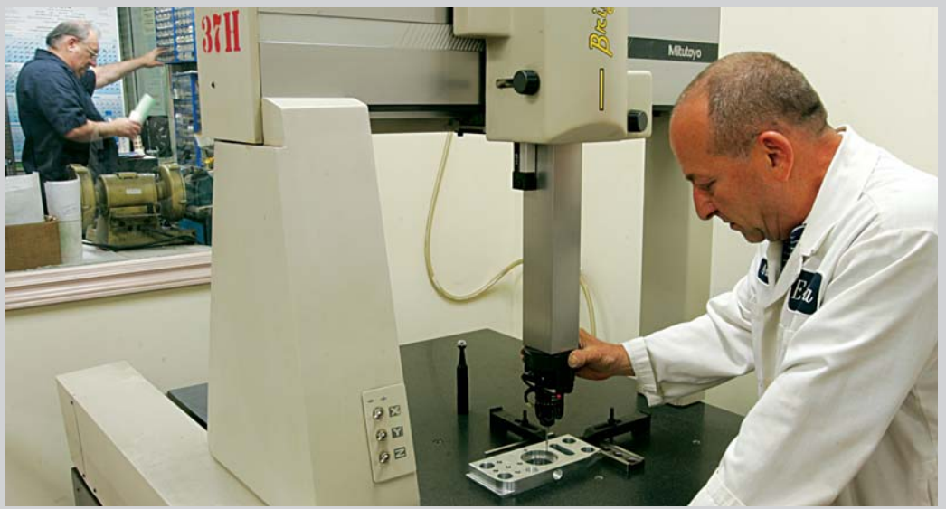
CNC Mitutoyo Co-ordinate Measuring Machine (CMM).
