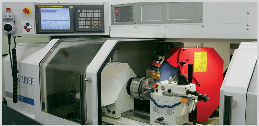
Studer universal grinder for high precision, O.D. and I.D. grinding.
