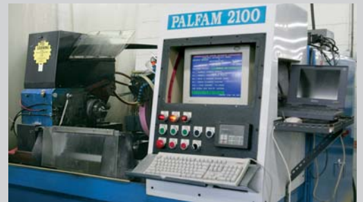
Custom built contour grinder for production runs of non round components.
