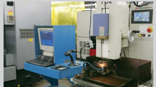
EDM drill capable of drilling .020 diameter holes through hardened steel.
