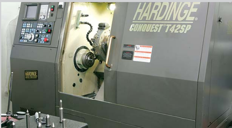
Hardinge super precision CNC lathe incorporates the latest technology for machining hardened steel.
