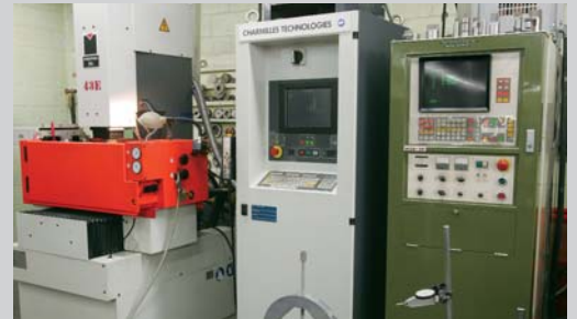
Charmilles sink type EDM with automatic electrode changer.
