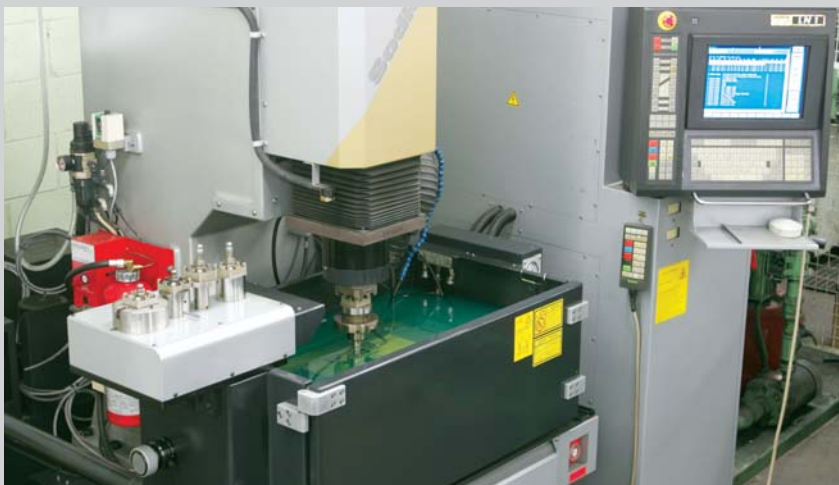
Sodick sink EDM complete with tool changer.
