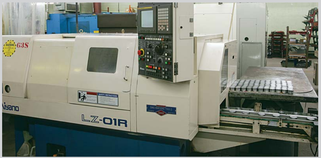
Miyano automatic self loading CNC lathe performs multiple operations for large or small quantity runs.
