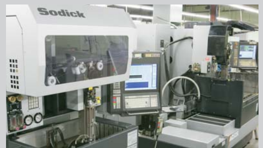
Sodick EDM with automatic wire threading for use on multiple cavities.
