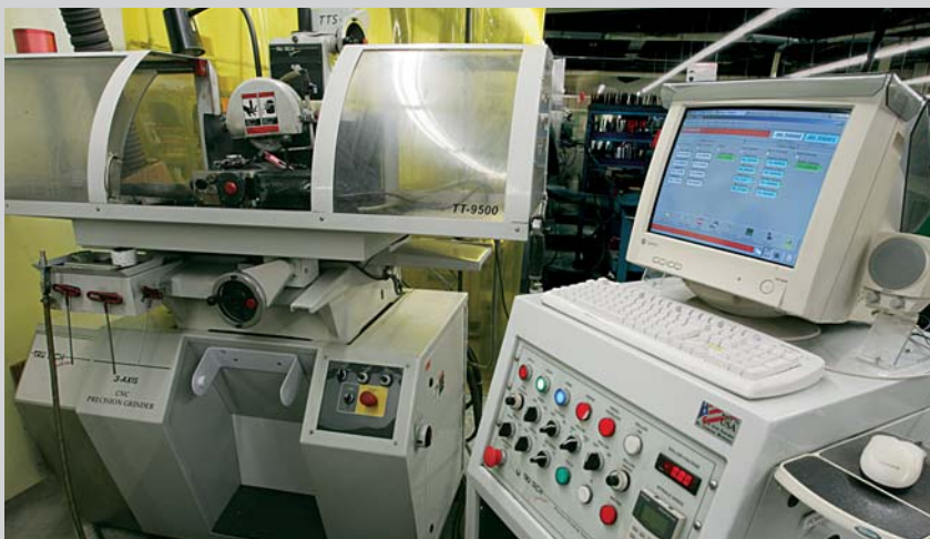
Tru Tech CNC grinder for small part production.
